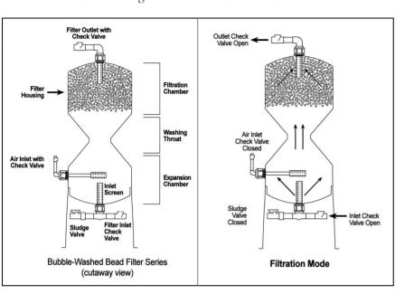
The floating nature of the beads and the bead size allows for simpler cleaning and less powerful pumps than used in e.g. sand filters. The inlet and outlet
