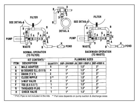
The pump assisted backwash can be combined with electrically actuated ball valves but extra equipment is needed. Please contact your local distributor for details.
