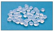
of the beads<sup>3</sup>. The very high surface area of the beads allows for the attachment of large numbers of beneficial filter bacteria, which break down fish wastes.
