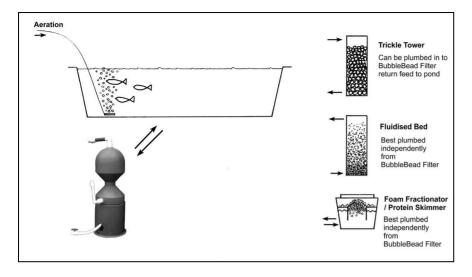
Foam Fractionators (Protein Skimmers) aid the removal of proteins and other surface active compounds from the water, reducing the load on other filter equipment and improving water clarity by removing staining compounds. Although foam fractionators show some benefits in freshwater, they work most efficiently on marine systems. They are not intended to remove solids from the water.
