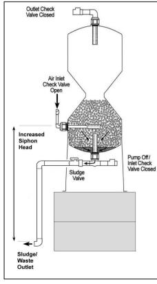
adding an extension pipe, the siphon head is increased and the efficiency of backwash greatly improved.
