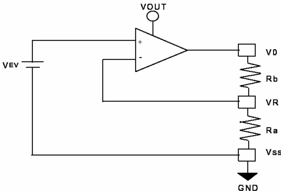
Figure 4. Internal Voltage Regulator Circuit
