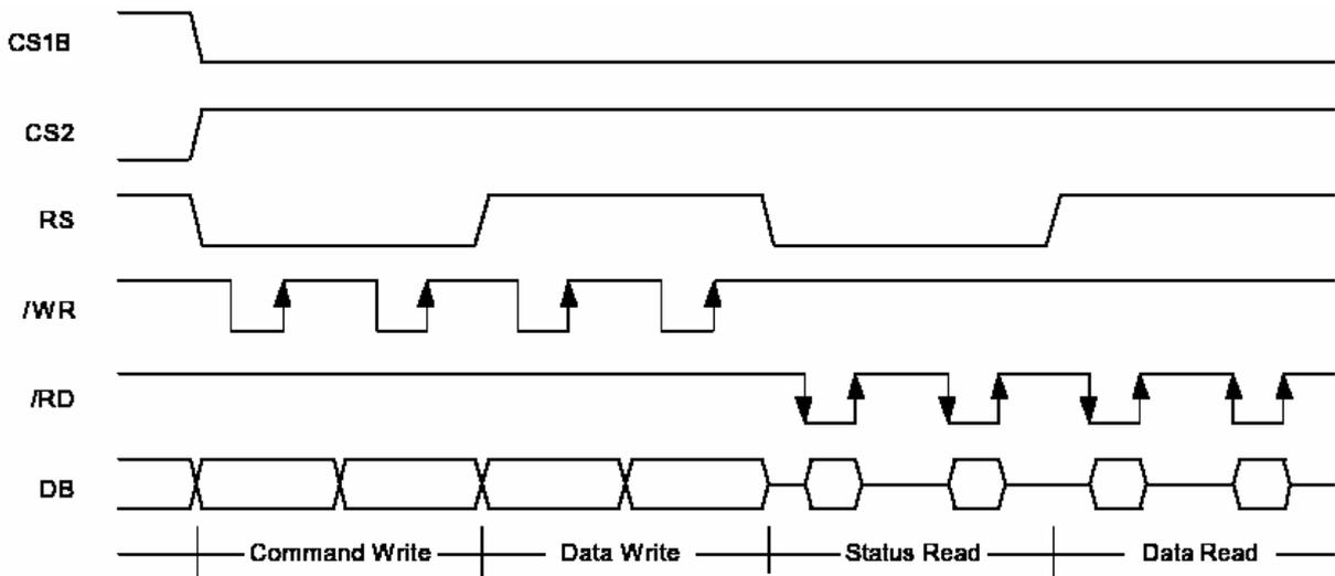
**Figure 2. 8080-Series MPU Interface Protocol (PS="H", MI="L")**
