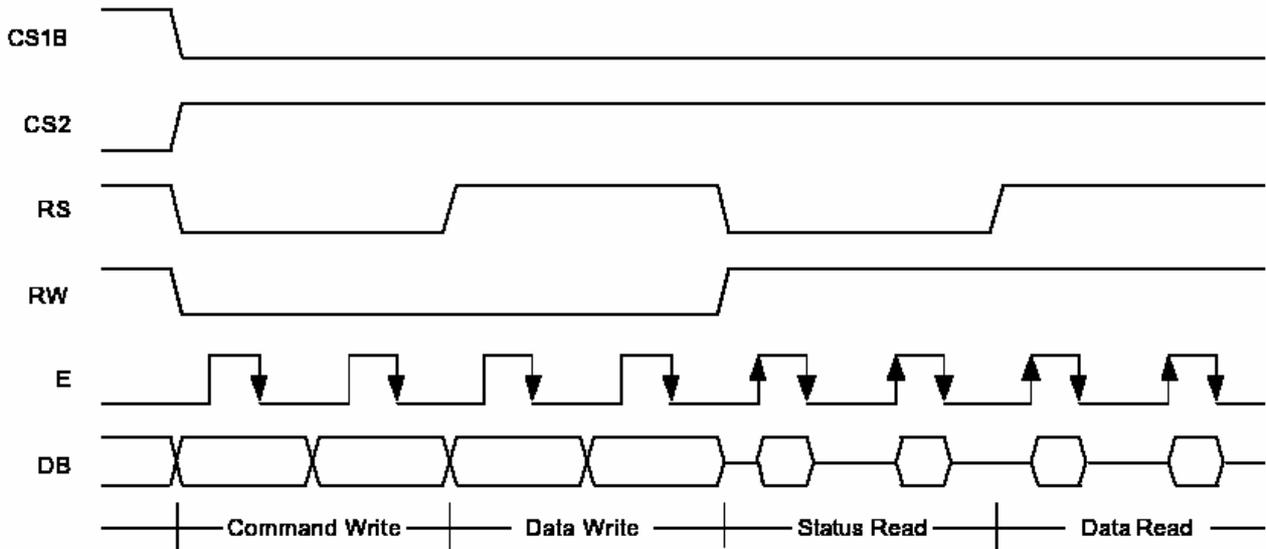
**Figure 1. 6800-Series MPU Interface protocol (PS="H", MI="H")**
