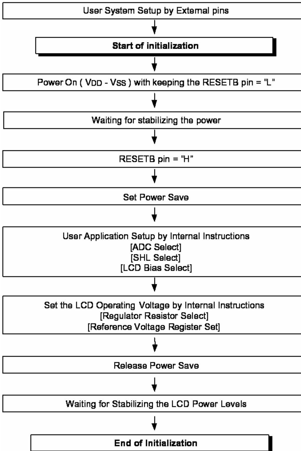
Figure 15. Initializing without the Built-in Power Supply Circuits
