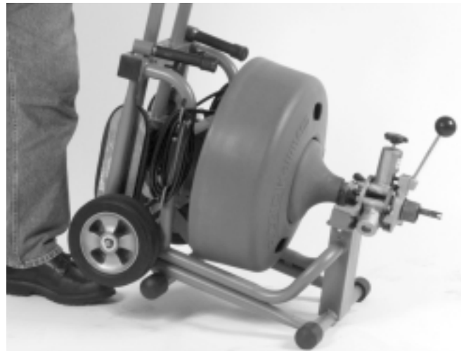
Figure 7 – Releasing Kickstand Bar
