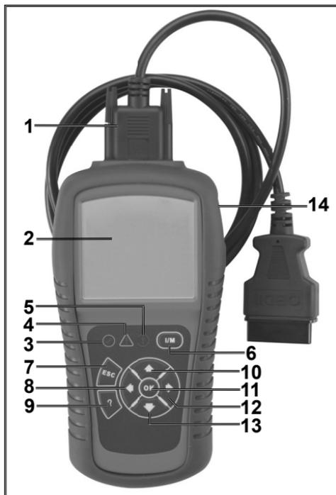
1. **OBD II Connector** – Connects the Scan Tool to the vehicle's Data Link Connector (DLC).
