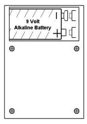
$\boldsymbol{Battery\ Compartment}$  - Install 9-volt battery into battery compartment as shown.
