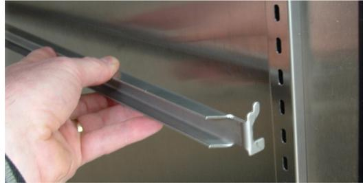
4. Slide each wire shelf into the corresponding pair of tray slides.
