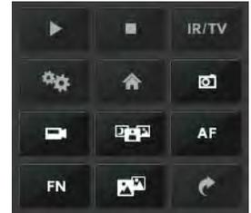
A disabled button is indicated with a grey color and when the cursor is over a disabled button, the screen tip indicates the function is not available. The disabled buttons correspond to commands that are not used with a fixed camera, but might be used to control a pan/tilt camera with multiple sensors.
