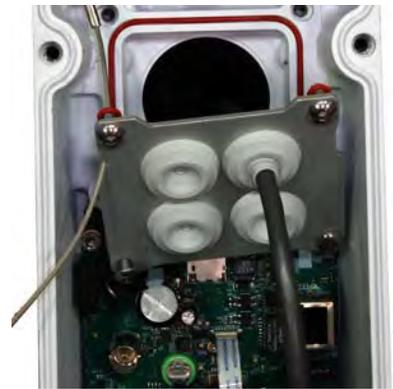
Figure 1-16: Cable through Seal Plate
