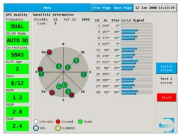
Each visible satellite is represented in the plot by a circle with the satellite ID number inside. All satellites used to compute the PVT solution are identified as
