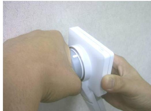
Step 3: Rotate and fasten Optical Lens in a counter-clockwise direction, where as the “Deco Ring” is at the “Horizontal” direction.
