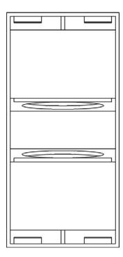
The G218B is the largest subwoofer in the G-Series, designed to offer the ultimate in low frequency reproduction. The G218B is designed to extend the low frequency performance of G12 and G15-based systems primarily, although it can also be used to support G8 and G6 systems in large installations. Through the use of a quasi-bandpass design, the enclosure size is kept to a minimum whilst still producing the required low frequency performance.
