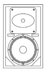
The G8 is a compact, fullrange loudspeaker. Contained within the sturdy Birch plywood enclosure is a powerful 8" LF driver and a 1" HF compression driver on a rotatable  $70^{\circ} \times 50^{\circ}$  horn. As with all G-Series fullrange enclosures, a G-Phase passive crossover network maintains flat frequency and phase responses whilst utilising the minimum number of amplifier channels.
