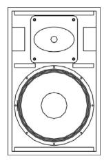
The G12 is a powerful, fullrange loudspeaker enclosure. Contained within the sleek enclosure is a 12" neodymium LF driver and a 1" HF compression driver on a rotatable  $70^{\circ} \times 50^{\circ}$  horn, matched by an internal G-Phase passive crossover network.
