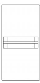
The G212B is a compact, powerful subwoofer system designed to extend the low frequency performance of G6, G8 and G12-based systems. Through the use of a quasi-bandpass design, the enclosure size is kept to a minimum to allow ease of use in installations where space is a premium.
