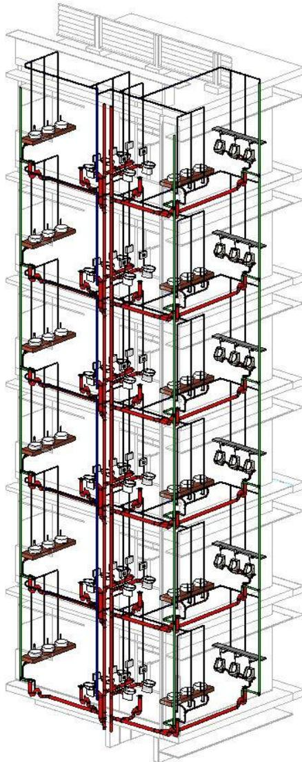
After Coordination, Copy the typical plumbing & sanitary routing to other typical floors and connect the riser to each other for it to become one connected piping system.
