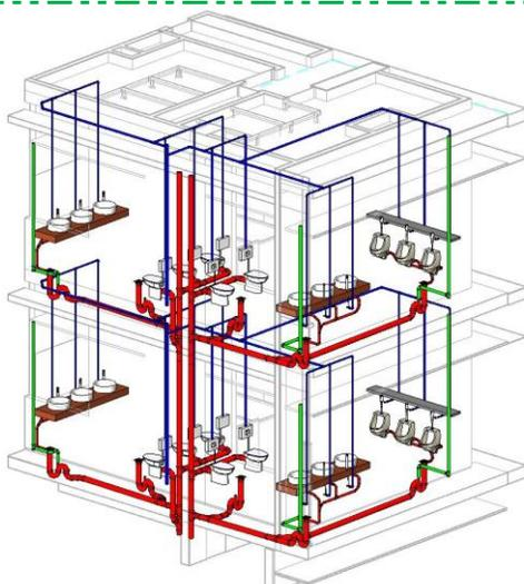
Typical Floor, Copy Plumbing & Sanitary routing to above level for further coordination.
