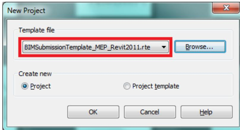
An example of MEP template can be found at <http://bimsg.wordpress.com/singapore-guide/e-submission/> . It is designed for MEP BIM e-submission.
