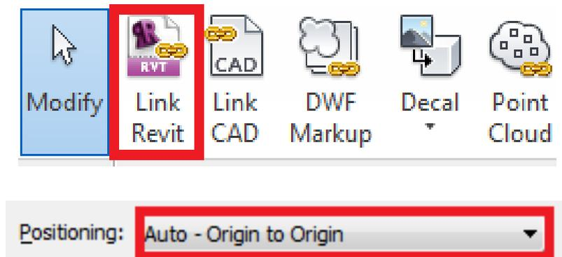
Note: Using Origin to Origin Positioning option to place MEP model at the same position as the Architectural model
