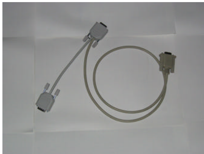
Picture 7 The serial cable splitter to provide both GPS and AIS data on one port.
