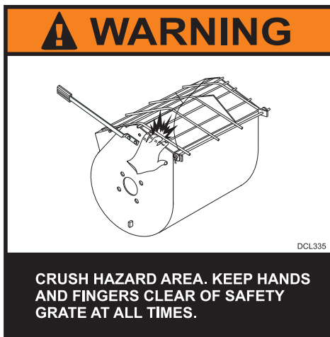
Figure 42. Safety Grate (Crush Hazard)
