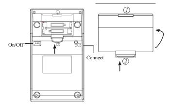
Snap the battery cover back into position.
