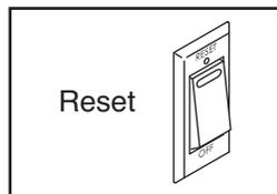
**IMPORTANT:** The console features a display demo mode, designed to be used if the incline trainer is displayed in a store. If the displays light as soon as you plug in the power cord and switch the reset/off circuit breaker to the reset position, the demo mode is turned on. To turn off the demo mode, hold down the Stop button for a few seconds. If the displays remain lit, see step 7 on page 21 to turn off the demo mode.
