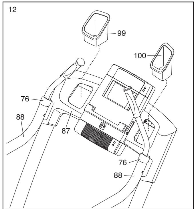
13. **Make sure that all parts are properly tightened before you use the incline trainer.** Keep the included hex keys in a secure place. One of the hex keys is used to adjust the walking belt (see pages 23 and 24). **To protect the floor or carpet from damage, place a mat under the incline trainer.**
