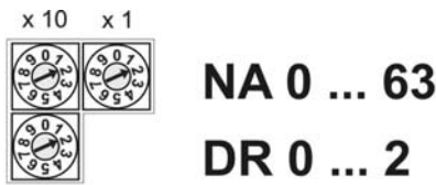
Fig. 23: Assignment of rotary switches for addresses and baud rate
