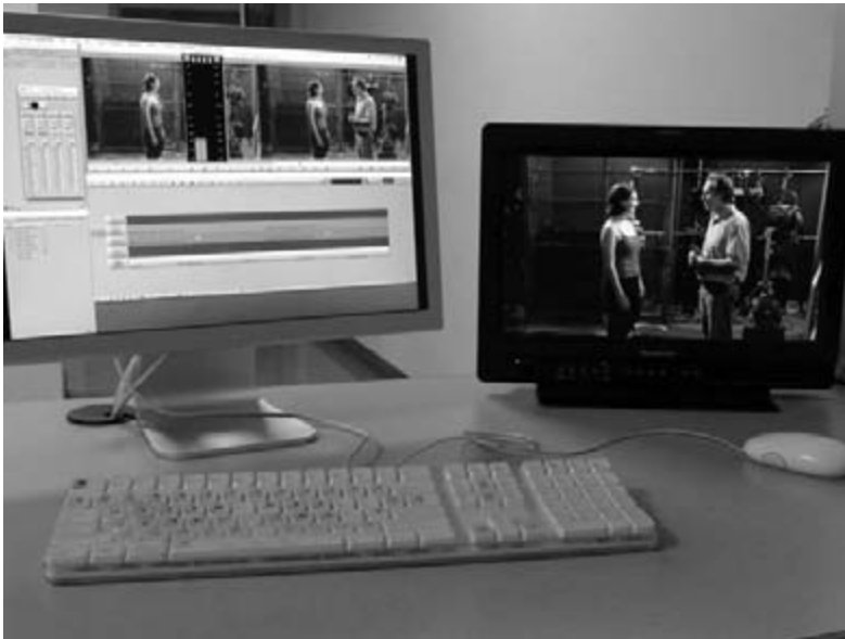
Figure 1.5 An Avid system with a high-definition client monitor.
