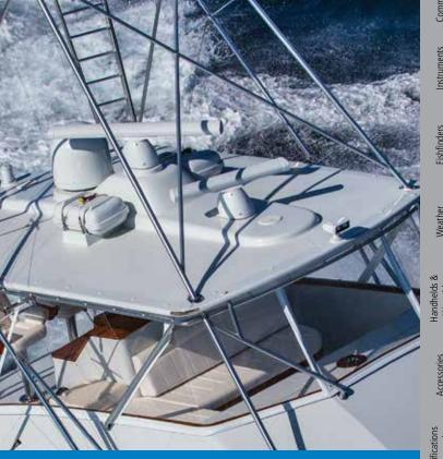
Garmin Shadow Drive technology provides the security of knowing you maintain control even when your autopilot is engaged. The Shadow Drive system automatically disengages the autopilot if the helm is turned, giving you the freedom to maneuver the boat. The autopilot automatically re-engages when you hold a steady course. Simple.
