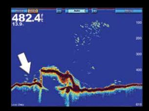
CHIRP has the sensitivity to differentiate between subtle differences to create a clearer image of what's
