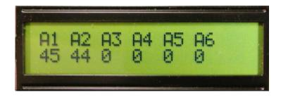
The second screen is shown above. This is the analog input screen. To verify proper operation of the analog inputs, use a cliplead to connect each of the analog inputs to +5v in turn. The screw on top of the terminal may not always make good connection until it is tightened, so don't be fooled until you know the connection is solid. Be careful not to touch the cliplead to the GND or REF terminals on the ends of the terminal block.
