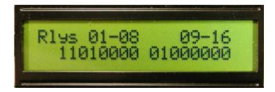
The same holds true for the relay screens. Above is the first relay screen. There are four, which display the relay status in groups of 16. We will return to this screen after the software is loaded.
