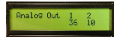
The next screen is analog out, shown above. The initial screen will be 00 for each output. The scale is rounded off again, with 50 representing 5.0vdc. The analog outputs can't be checked without the software to send commands, so we will skip this until we install the software and are ready to check it.
