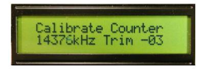
The final screen is the counter calibration screen. This is required because I chose to use a ceramic resonator for the PIC clock to avoid problems with isolation between the high gain counter preamp and an external xtal oscillator. The counter is not meant to be a precision instrument, only a way to verify that you are transmitting on the frequency that you think you are at the remote site.
