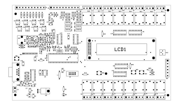
Parts can be assembled in any order, but I recommend installing the DIP sockets first so that the board can lay flat during their installlation. Next I would install the tactile switches and LCD socket, so that they can be held firmly against the board while soldering them.
