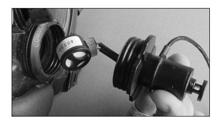
• Unscrew the communication port plug; insert the microphone through the port into the mask with the hydrophobic membrane facing the visor.
