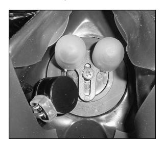
• If the membrane is turned the wrong way, facing the mouth, phonic performance will be diminished. Move the microphone so that it does not interfere with the diver's lips or the pressure equalization system.
