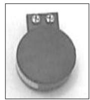
The GSM DC use a dynamic microphone, "D-Mic" encapsulated and protected by a hydrophobic membrane.
