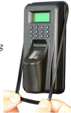
8-5: Installation of silica gel strip
