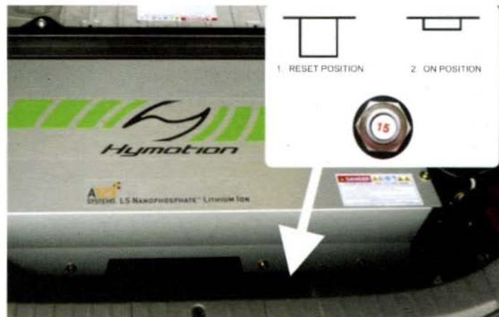
Figure 7 L5 PCM circuit breaker
