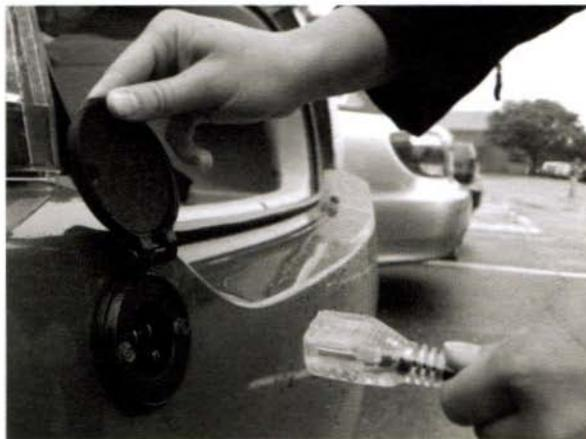
Figure 5 L5 PCM charge port location
