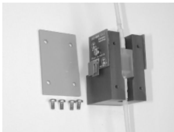
Figure 12.2.2: Body Assembly and flow cell
