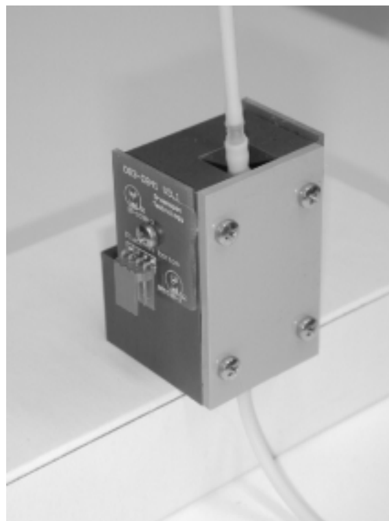
Figure 12.2.1: Phosphate body assembly
