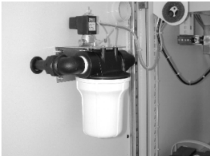
Figure 12.1.6: The sample delivery module
