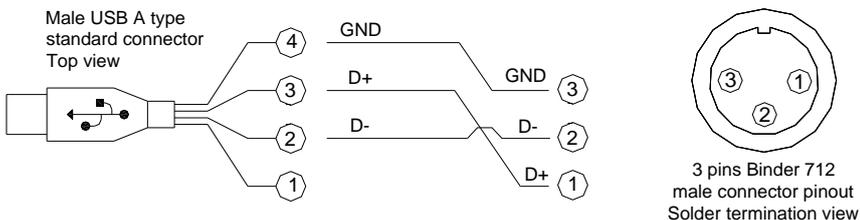
USB male connector pinout
