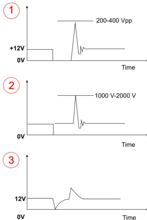
**It is reminded that the adapter white cable, labelled "RPM-Coil 150-400 V" is to be connected to the RPM trigger wiring indicated by digit 1 in the above schemes.**
