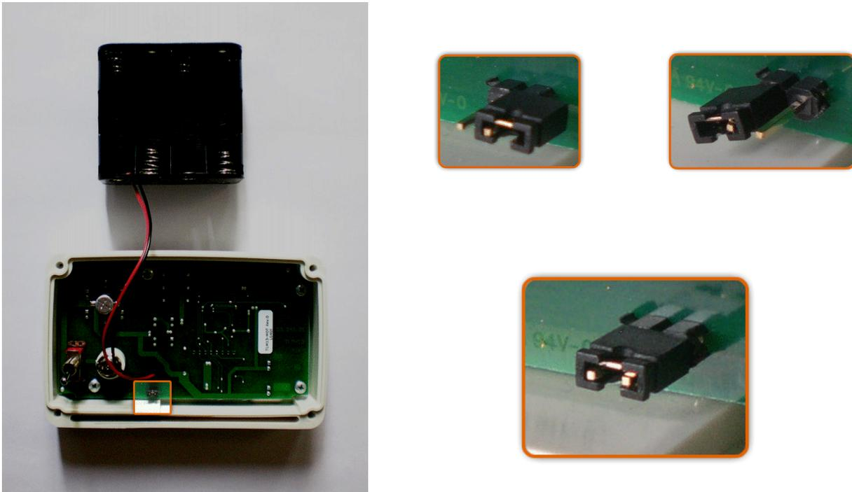
The image here above on the right shows possible working mode. The transmitter comes set in low power mode: see images top on the right. To set high power mode insert both clips in the jumper: image bottom on the right.
