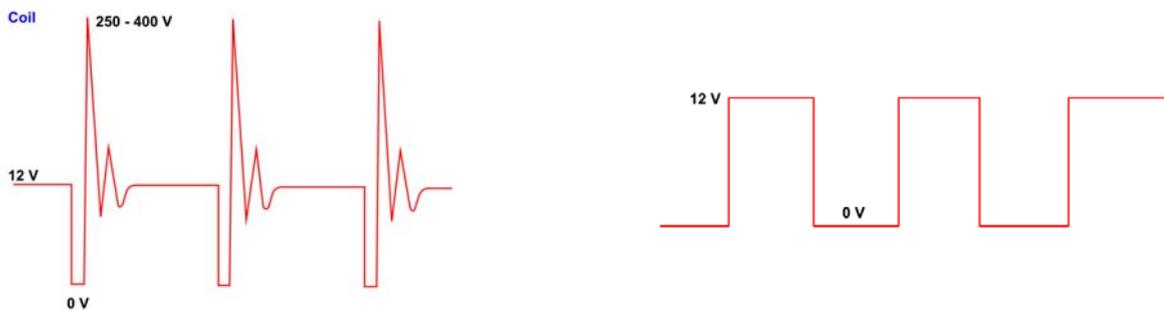
To filter the signal use an “RPM Coil-ECU” adapter (optional). It is a double-purpose filter that allows to sample RPM from the coil and squares the signal wave form.
