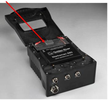
When the *Marksman 680* is installed in an equipment cabinet, mains power will usually be available to keep the main battery fully charged, using the Battery Charger GR006830/6831 (Section 5.4). In such an installation, the only purpose of the main battery is to ensure continuity of data collection during mains outages (which are expected to be repaired long before the capacity of the battery has been exhausted).
