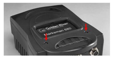
2. Stand the *Marksman 680* on its base as shown above, and unfasten the two screws in the lid (arrowed in red) until the lid can be lifted. The lid will then hinge backwards to reveal the battery.
