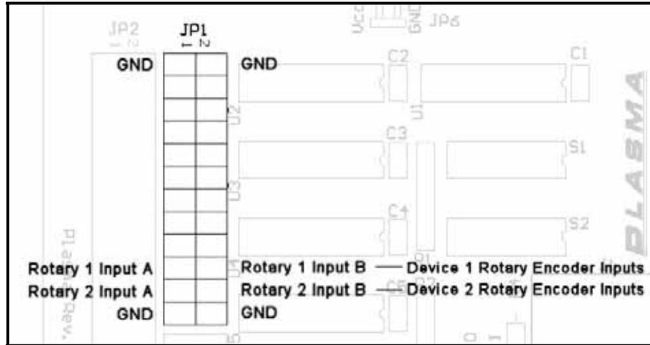
The mechanical rotary encoder inputs convert 2-bit gray code type encoders only. These inputs are buffered to prevent lost inputs with a maximum output rate limited to 12 PPS (Pulses Per Second). The pulse output is comprised of a 40 ms ON pulse followed by a 40 ms OFF pulse.
