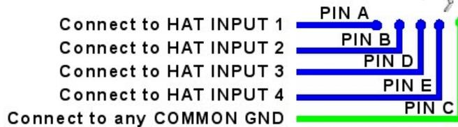
The POV HAT switch common pin must be connected to one of the ground pins. All other HAT switch pins must be connected to the appropriate input pins as describe above.
