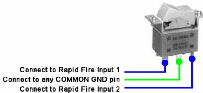
Inputs 1 & 2 can be wired to a momentary rocker switch (MOM-OFF-MOM) for use as a digital trim switch.
