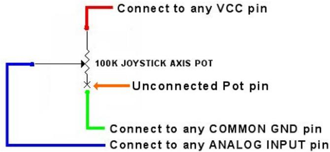
NOTE: Conventional analog Joystick potentiometers have one unconnected pin on axis pots. It is imperative that this pin be grounded in order to properly function when connected to the Plasma analog port inputs.
