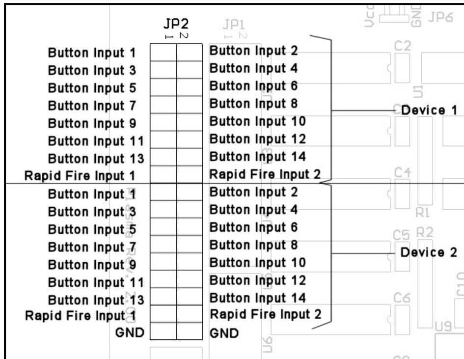
Unlike the standard button inputs, *Rapid Fire Inputs* send a pulse stream instead of a continuous ON signal. The pulse rate has been preset to 10 PPS (Pulses Per Second).
