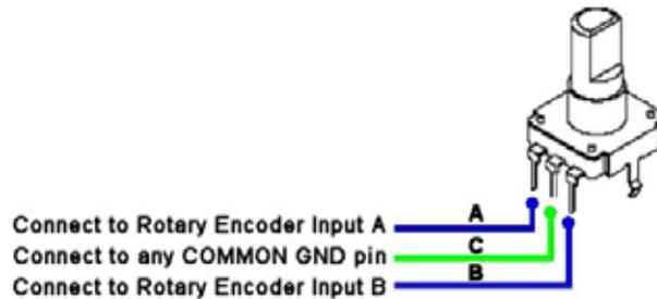
Rotary outputs are located on button inputs 17 & 18 in MODES A & B (figure 4) and button inputs 31 & 32 in HOTAS MODES C & D (figure 5).
