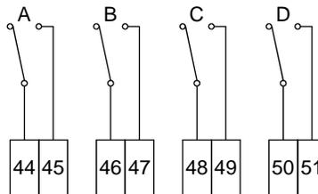
Figure 9.10 PR-7080 Relay output connections. In wash control relay unit-WR only A and B available.
