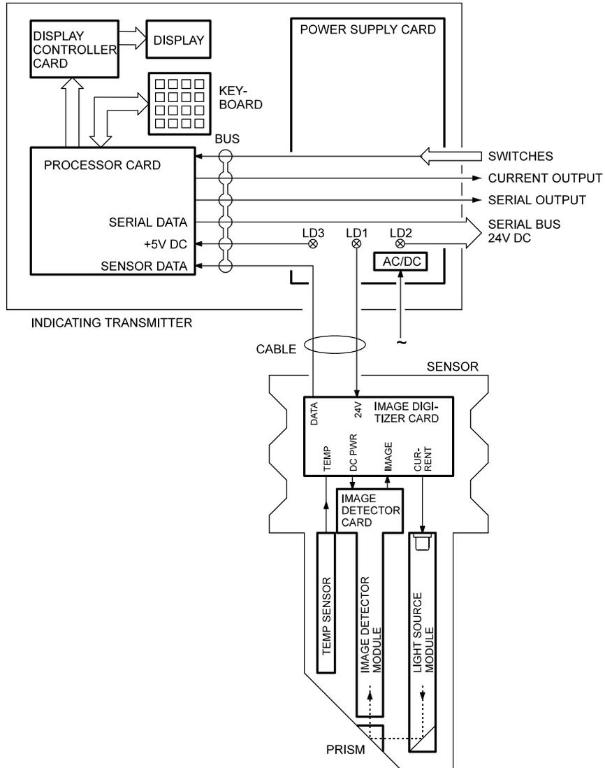
Figure 6.21 Information and power flow. For intrinsically safe system, see Figure 12.50.
