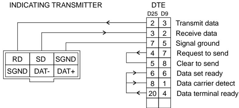
Figure 3.71 RS-232 connection to DTE-type equipment (e.g., computer).
