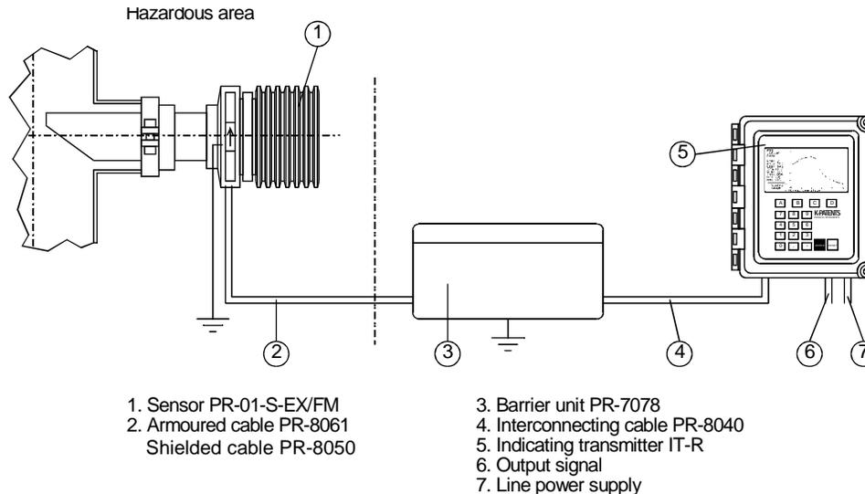
Figure 12.10 Intrinsically safe equipment.
