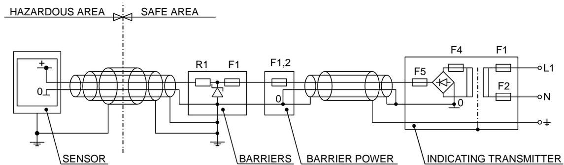
Figure 12.51 Earth connections.
