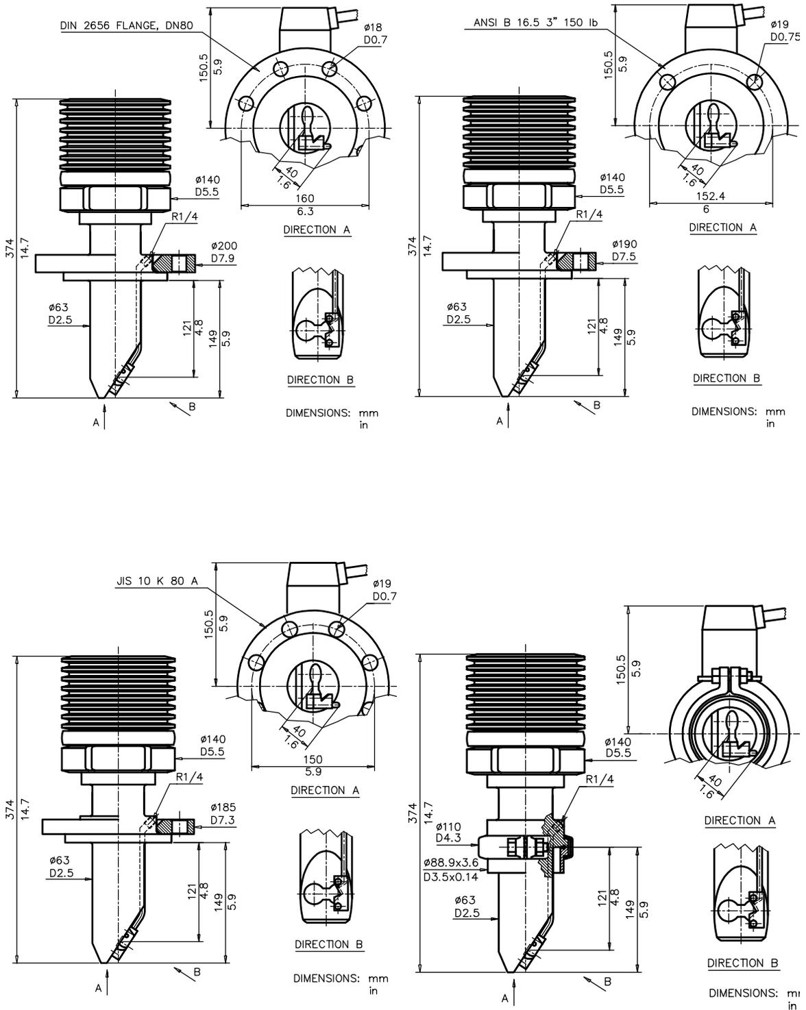
Figure 8.21 Mounting of integral steam nozzles with DIN, JIS, ANSI and Sandvik connections.
