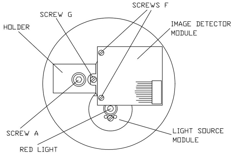
Figure 6.80 Sensor: Image Digitizer Card removed.
