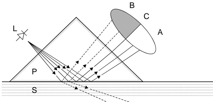
Figure 2.30 Refractometer principle.
