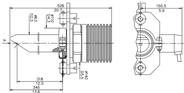
Figure 11.10 Model PR-01-S-LPH, Long Probe adapted to Retractor HIMP-2.
