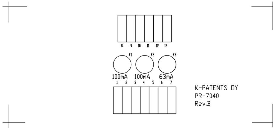
Figure 12.41 Barrier power card PR-7040, components lay-out.
