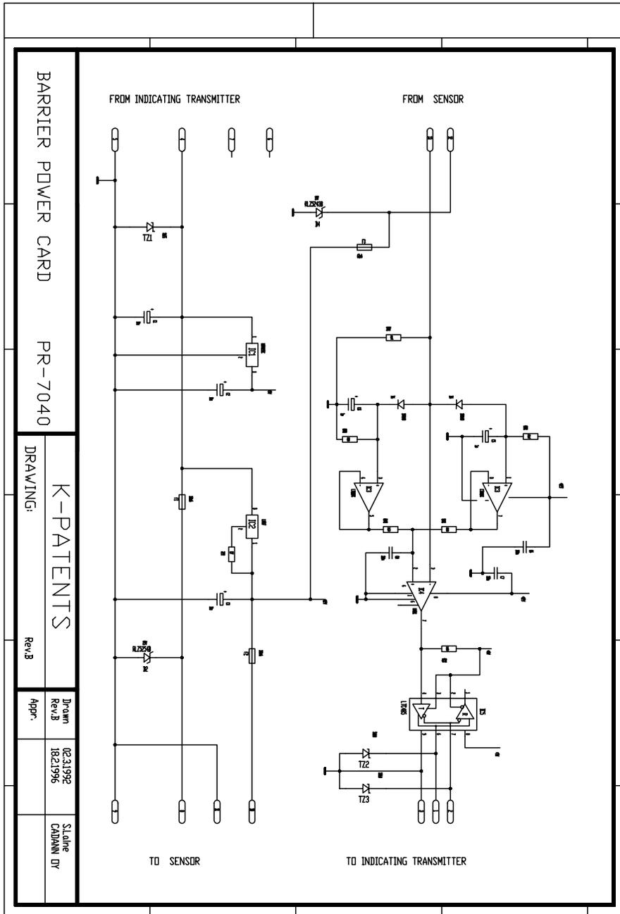
Figure 12.40 Barrier power card PR-7040, Circuit diagram.
