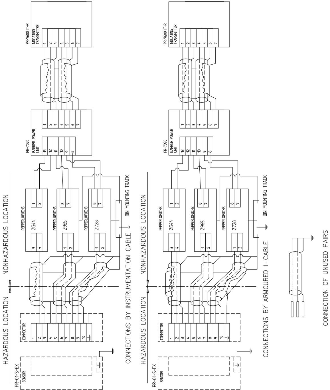
Figure 12.22 Intrinsic safety field wiring for PR-01-S-EX.
