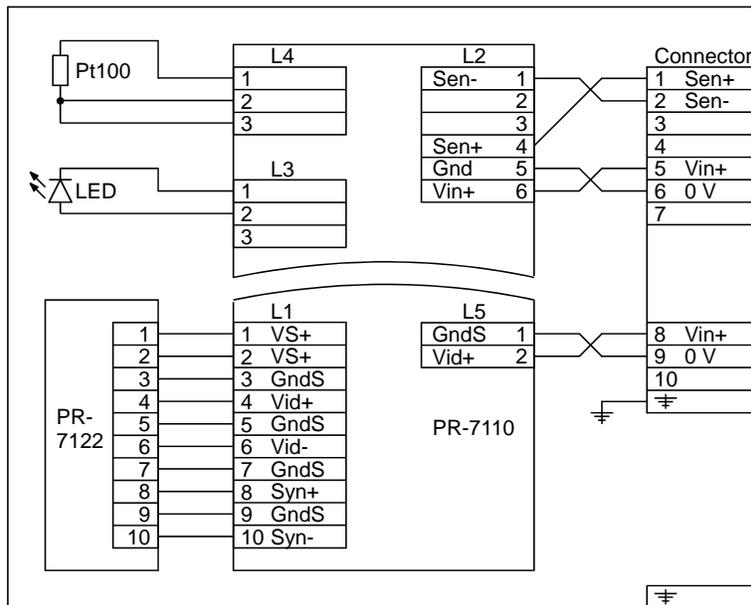
Figure 12.53 Intrinsically safe Sensor: Internal wiring.
