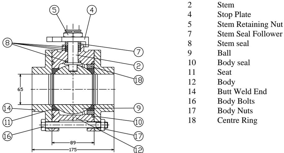
Figure 11.40 Ball valve parts list.
