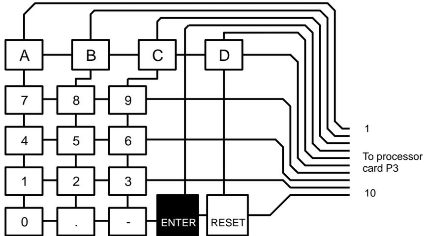
Figure 6.46 Keyboard switch matrix.
