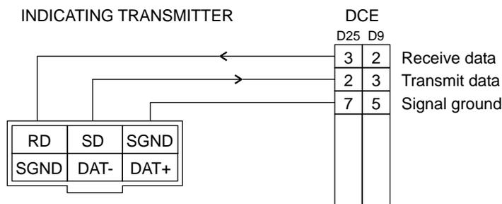
Figure 3.70 RS-232 connection to DCE-type equipment (e.g., modem).
