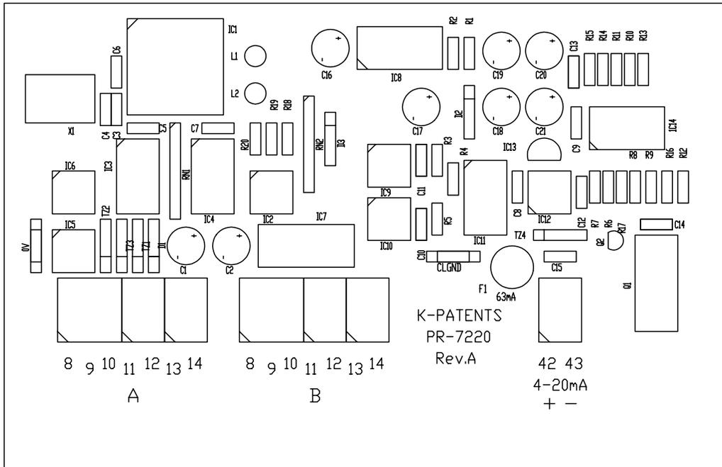
Figure 10.10. External output unit, component lay-out.
