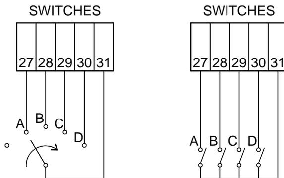
Figure 3.64 Connections to input switches.
