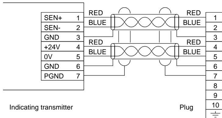
Figure 3.62 Interconnecting cable. For intrinsically safe systems, use Figure 12.22.
