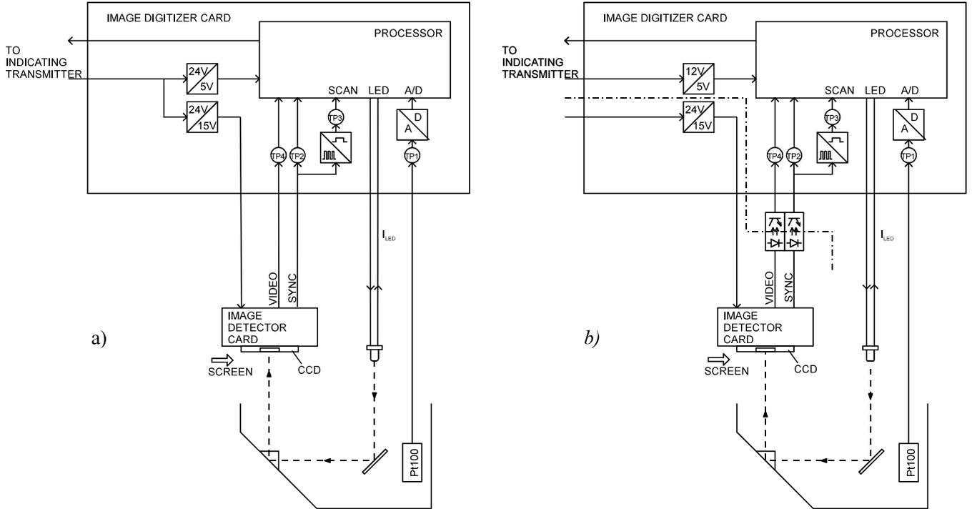
Figure 6.50 Sensor information and power flow.
