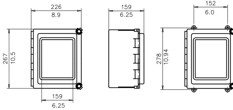
Figure 2.20 Indicating transmitter: Dimensions (mm/in) and mounting feet measures.
