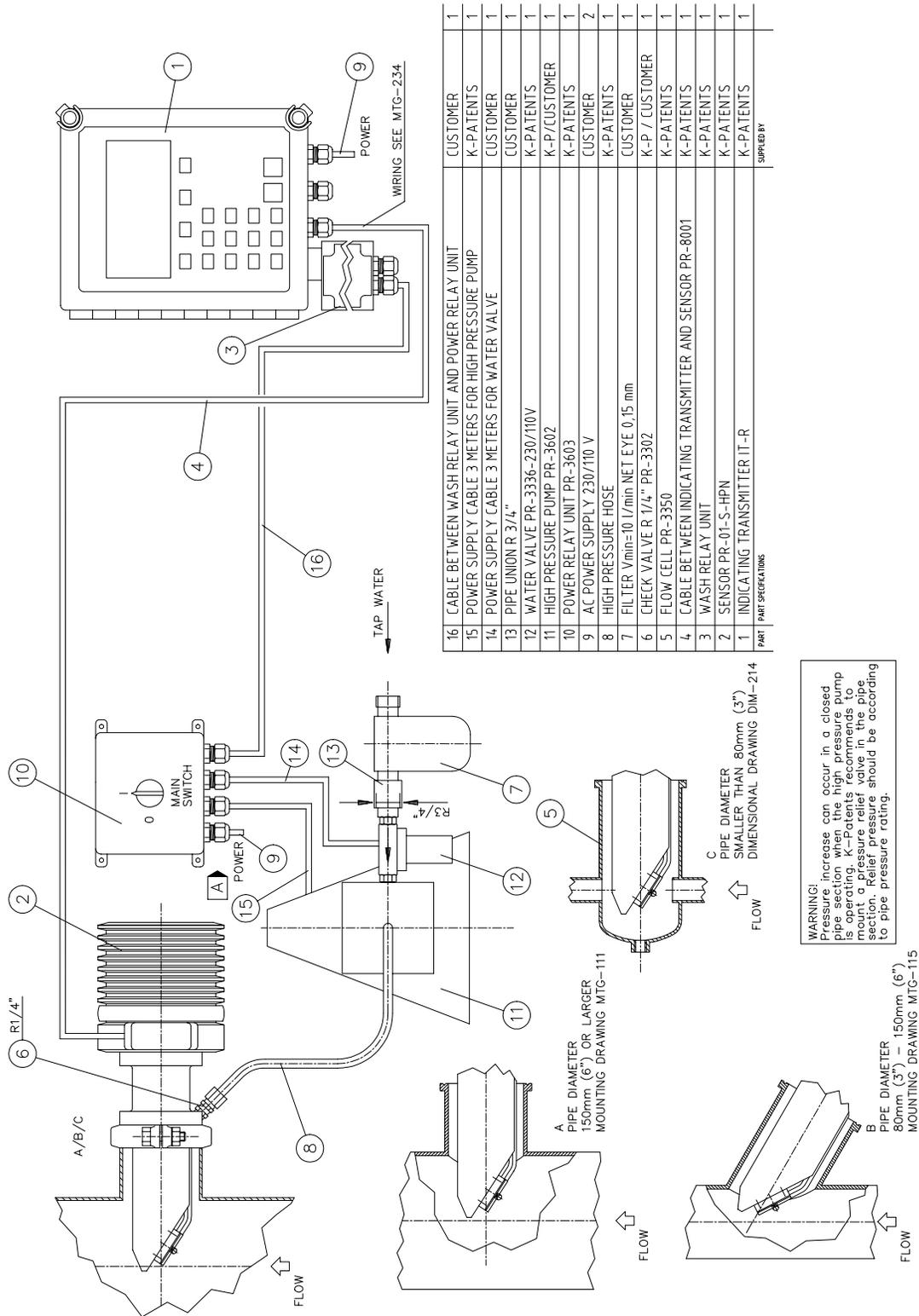
Figure 8.32 Mounting drawing for integral high pressure wash system with Wash control relay unit - WR.
