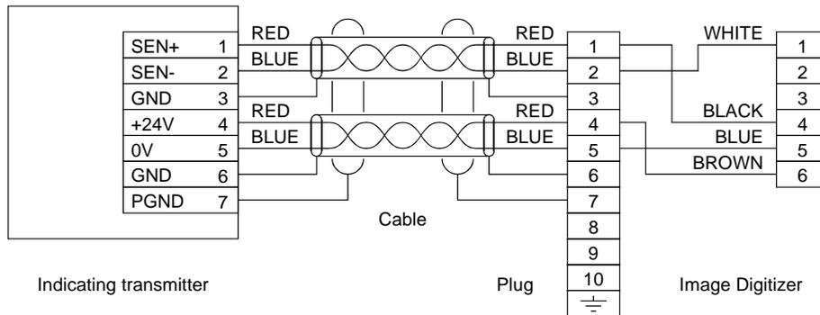
Figure 6.22 Cable signals. For intrinsically safe systems, use Figure 12.22 (field wiring) and Figure 12.53 (internal wiring).
