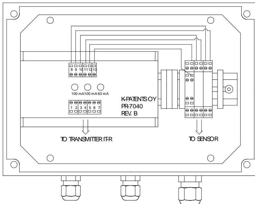
Figure 12.30 Mounting of barriers and accessories.
