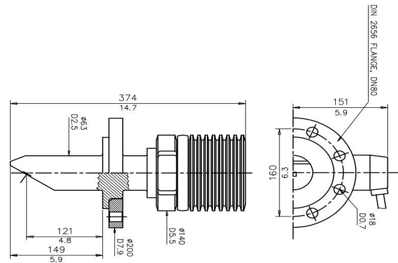
Figure 2.22 Dimensions: Sensor with flange. DIN 2656 DN 80 or ANSI B16.5 3" RF 150 PSI or JIS 10K 80A (mm/in).
