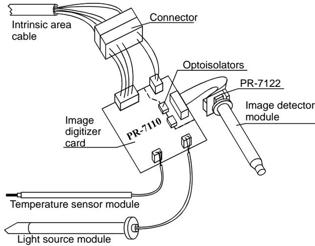
Figure 12.52 Intrinsically safe Sensor: construction of the electronics.
