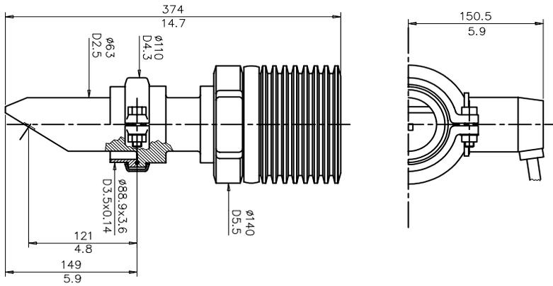
Figure 2.21 Dimensions: Sensor with Sandvik clamp (mm/in).
