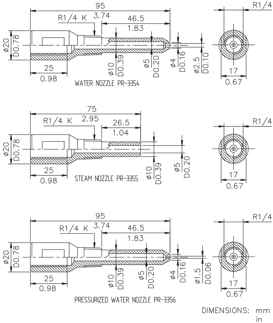
Figure 8.41 Flow through cell nozzles.
