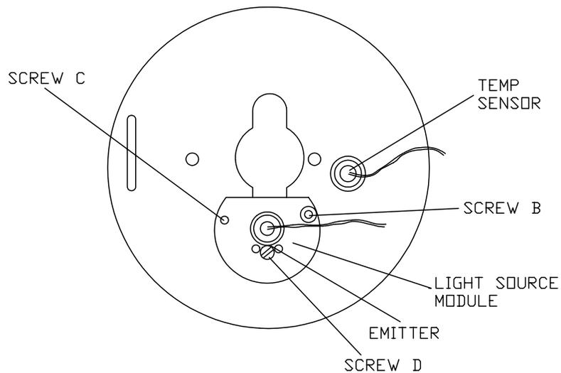
Figure 6.81 Sensor: Image Detector Module removed.
