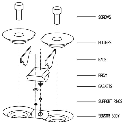
Figure 6.70 Prism mounting.
