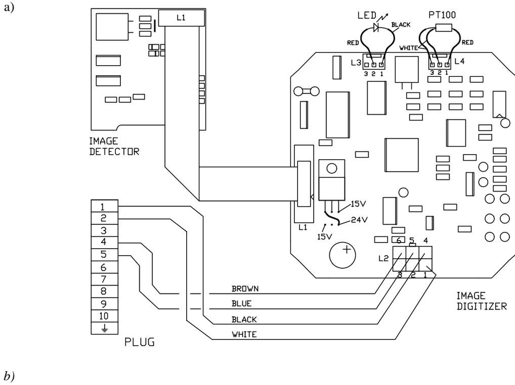
Figure 6.52 Sensor electronics test points.
