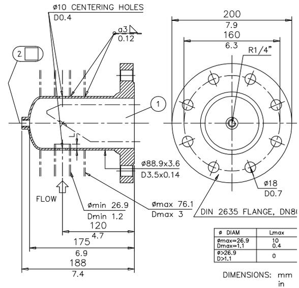
Figure 3.21 Flange mounting DIN 2635 DN 80. Note for ANSI B16.5 3" RF 150 psi or JIS 10K 80A separate drawings are provided.
