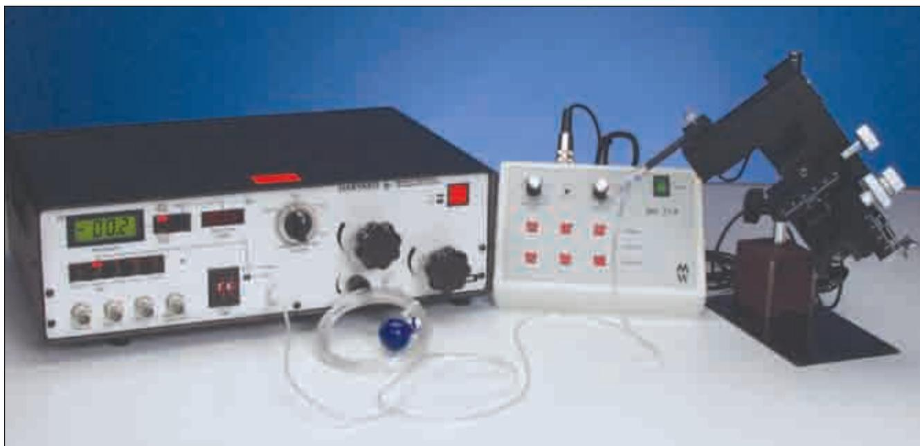
The PLS-1 Pico Injection/Micromanipulator System combines our popular PLI-100 pico injector, a motorized micromanipulator, and magnetic base in a single package.
