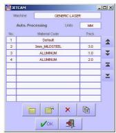
do that by indicating a material and clicking the EDIT button. Use the COPY command to speed up the setup process. The highlighted material will be copied (including all setup parameters). This will save time when creating materials which will have similar setup parameters to existing ones (and usually, all you will have to do is specify a new material type and thickness for the copied material entry). You can then use the EDIT command if you need to modify any values for the new material.
