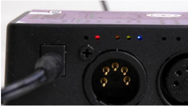
DMXioR3 LED indicators use blink patterns to indicate various settings.
