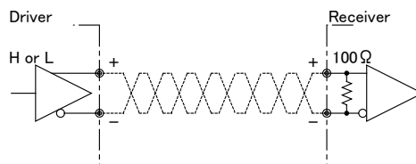
Figure 3-3-2 Circuit of LVDS
