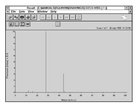
Characteristic spectrum of carbon monoxide and carbon dioxide outgassed by filaments and ion source. Solve by switching quadrupole into degas remembering to degas filaments of other equipment such as ion gauges.
