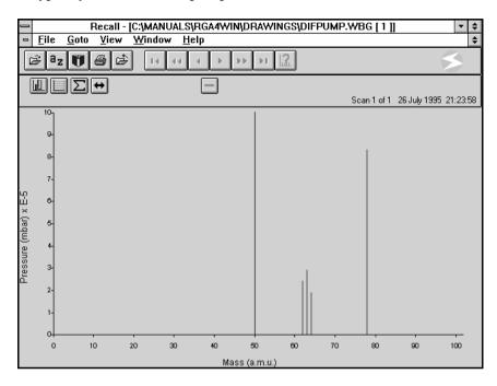
Characteristic of spectrum of polyphenylether diffusion pump oil. Solve by fitting efficient baffle or cold trap and bake.
