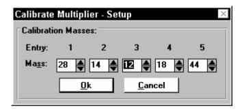
If the masses listed do not suit your vacuum system they may be changed either by typing in a new value or by *clicking* on the spin buttons. The masses used in calibrate may be set to any mass within the mass range of the instrument.
