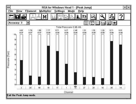
Peak Jump has two display modes. The results may be plotted on either a Logarithmic y-axis with a selectable number of decades or on a linear y-axis showing the results in the range 0.00 to 9.99. When Logarithmic mode is selected, autorange is automatically enabled for all channels. This allows partial pressures to be measured and stored over the full range of the selected detector, while only the decades of immediate interest are displayed.
