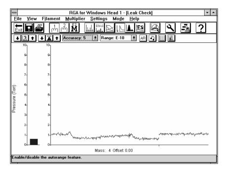
The second use of Leak Check is as a general purpose monitor of single peak height with either very fast response or very stable readings.
