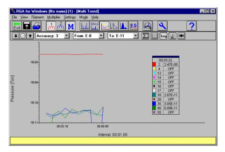
You have the option of a logarithmic intensity scale. This enables you to display trends over the full dynamic range of the instrument, and is probably the most widely used mode for general process monitoring.
