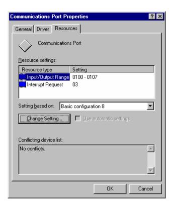
5) Change the Setting <u>based</u> on: setting to 'Basic configuration 8'. Once this is done you will be able to change the Input/Output Range (Base address) and Interrupt Request (IRQ) settings by *double clicking* them and selecting the appropriate values for the configuration of your comms card.
