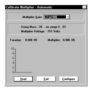
The current voltage applied to the multiplier, and the first mass in the mass list that will be used for calibration are shown.
