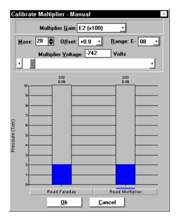
The multiplier gain can be selected from the **Multiplier Gain:** *dropdown list*. The required mass for the calibration can be typed in the **Mass:** box or entered using the spin buttons. As with the Leak check mode the mass can be fine tuned by selecting a valve between +0.5 and -0.47 from the **Offset** *dropdown list*. The range for the calibration can be selected from the **Range E**- *dropdown list*. This should be selected so that the faraday reading is in the range 0.9 to 9.0.
