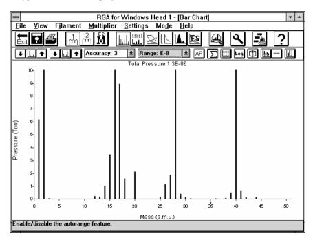
This mode allows one of a number of pre-set ranges of consecutive masses to be scanned. The starting mass (First mass) can also be specified. This
