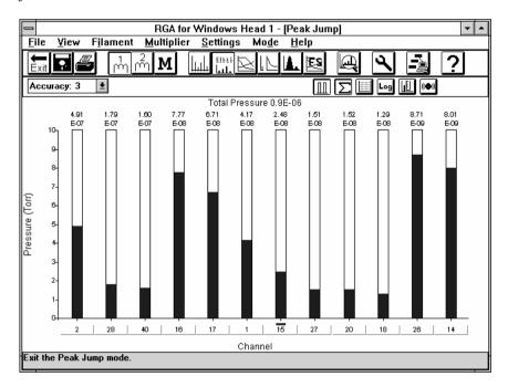
This mode enables you to individually set the mass in any of the twelve channels. You can assign each individual channel to either a specific gain range or, set the instrument to autorange throughout its whole dynamic range. This gives tremendous flexibility for process monitoring as you can monitor high and low level components simultaneously. As you are only
