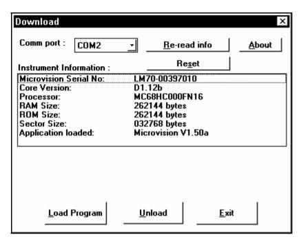
Select the comm. port by *clicking* on the **Comm port**: *dropdown list box* and then *click* on the required comm. port. As soon as you do this the RGA for Windows software will try to establish communications with the control unit. If this is successful one or more lines of information will appear in the **Instrument Information:** box. This process can be repeated by *clicking* on the **Re-read info** button and will be repeated each time a new comm. port is selected.
