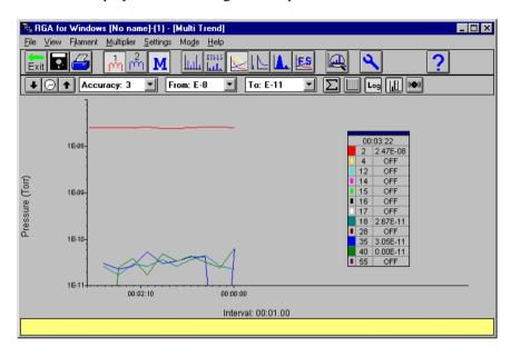
Multi Trend has two display modes. The results may be plotted on either a Logarithmic y-axis with a selectable number of decades or on a Linear y-axis showing results in the range 0.00 to 9.99.
