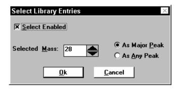
Select Library Entries operates as a filter on the library entries, initially 62 spectra. With select disabled all 62 entries are available and Carbon Dioxide for example will be displayed as (12 of 62). With select enabled only spectra containing a chosen mass or a chosen mass as the major peak will be available
