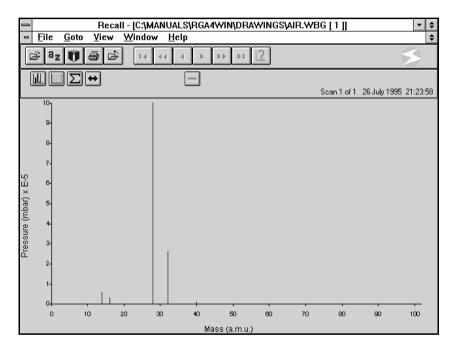
Characteristic spectrum of an air leak, masses 28 and 14 from nitrogen, 32 and 16 from oxygen, 40 from argon.
