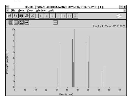
Characteristic spectrum of rotary pump oil contamination, due to foreline trap not fitted or in need of reactivation. Solve by fitting or reactivating trap as appropriate and bake vacuum system.
