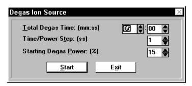
The **Time/Power Step:** (ss) is the time, in the range 1 to 59 seconds, spent at each power level. There are 256 power levels within the range of 15% to 100% of full power.
