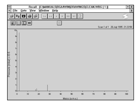
Characteristic spectrum of a clean high vacuum. Note the relatively high level of hydrogen which is desorbed from the metal walls of the vacuum system. Mass 28 due to carbon monoxide will always be present, the extent depending on how many filaments, and their types, are in operation.
