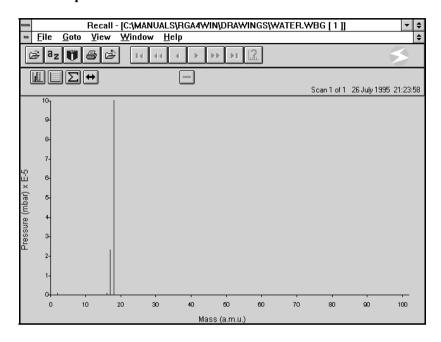
Characteristic spectrum of water vapour in the vacuum system. The problem is solved by baking the system to 250 deg. C for some hours, preferably with an oven to ensure a uniform baking temperature. Remember to avoid sudden large temperature changes on ceramic and glass components to prevent damage.
