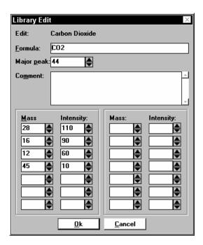
All of the entries may be edited except for the name (Carbon Dioxide in the above graphic). Position the cursor in the appropriate box and type the required value or text or use the *spin buttons*. Once you have completed the changes click on the  $\mathbf{Ok}$  button.
