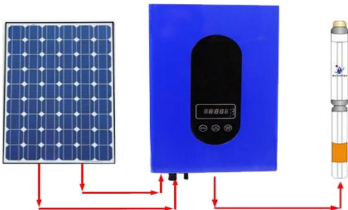
Solar pump system mainly including 4 parts: Solar Array, solar pumping inverter, AC pumping and water storage device. This system can solve the demand of water supplying issue in powerless area and improve their living and production status.
