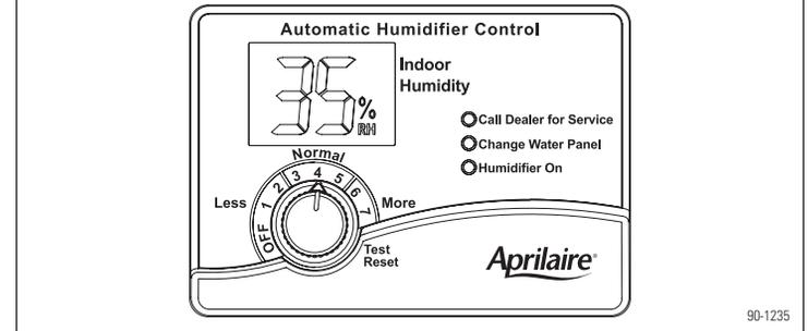
Your Aprilaire Humidifier Control is installed in the cold air return duct. **During the first heating season**, your Humidifier Control needs to be set initially to match your home's condition. Please follow these steps when adjusting your control (refer to **Figure A**).
