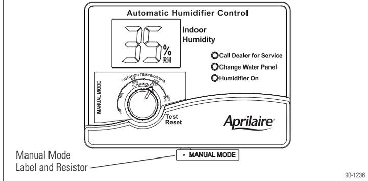
When installed in the Manual Mode (see **Figure B**), it is important to anticipate a drop in outdoor temperature and reduce the setting accordingly to avoid excessive condensation. For example, with an outdoor temperature of 20°F the correct setting will be 35% RH. If the temperature is expected to fall to 0°F that evening, then merely reduce the setting to 25% several hours prior to the temperature change.
