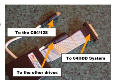
If you have a serial pass-through port on your cartridge then that needs to be connected in-line with the cables going to your drives. Connect one end to the C64/128 and connect the other end to the serial cable leading to your other drives or XE1541 cable (if you have no other drives then it is Ok to leave this end disconnected).
