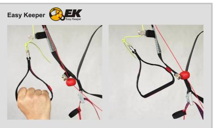
Easy Keeper is our indigenous way to hold the brake handles at the risers by using strong neodymium magnets. It keeps the handles firmly at the risers, while both attaching and releasing goes smoothly and easily. The system allows for easy placing the brake handles on risers during flight, when they are not used, thus minimalizing danger of getting them into running propeller.
