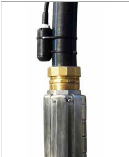
Figure 22: Well probe fixing
