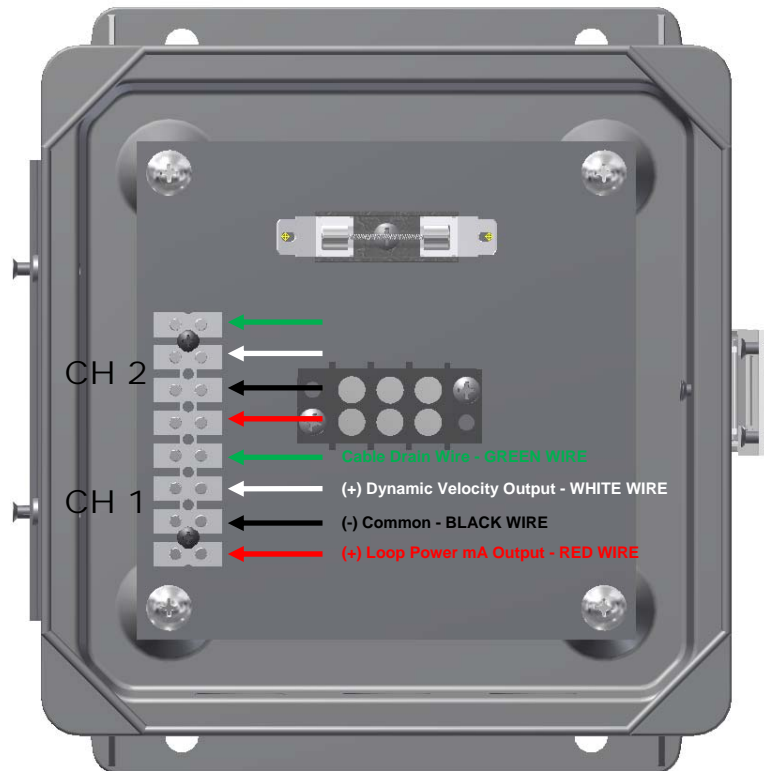
Figure 8 - PMX3000 Series System Input Wiring
