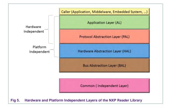
host. Therefore, the developers can use them seamlessly with any communication interface supported in the Bus Abstraction Layer (BAL).
