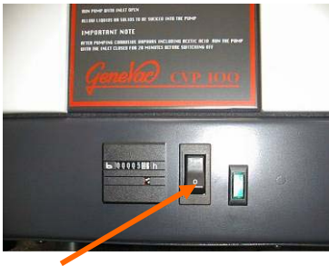
CVP pump power switch
