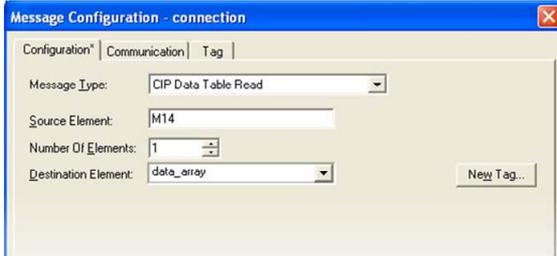
Figure 95: Read the Inverter's Operation Status Register
