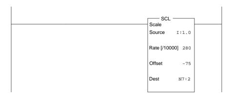
Examine the parameters entered into this SCL instruction, and then calculate the actual integer value written to N7:2 at a temperature of 100 degrees F (4 mA signal) and the actual integer value written to N7:2 at 800 degrees F (20 mA signal). The results will *not* be exact due to rounding of the Rate and Offset parameters.
