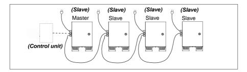
Set the light generator as Master by setting the code wheel 3 to "9".
