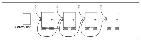
If there is more than one light generator they must be connected in a daisy chain connection
