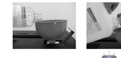
2.4 Pour the fuel to the point where the blue indicator blinks sound. Stop pouring! Remove the funnel.
