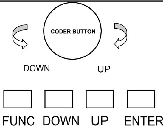
Projector configuration can be set conveniently via pressbutton switch and LCD display. Turn the projector on and the LCD display will show DMX address you set and save last time and it can be reset and saved again as you please.
