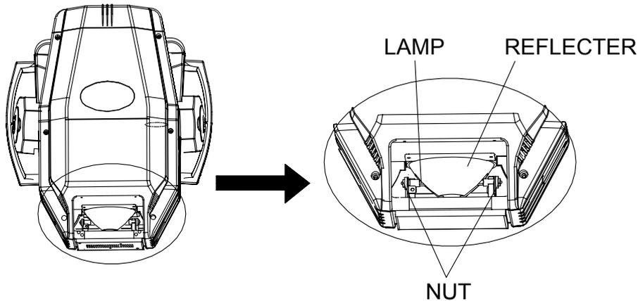
Lock the yoke before fitting/replacing the lamp.
