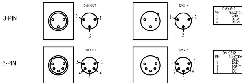
Connection between controller and projector and between one projector and another must be made with a 2 core-screened cable, with each core having at least a 0.5mm diameter. Connection to and from the projector is via cannon 3 pin (which are included with the projector) or 5 pin XLR plugs and sockets. The XLR's are connected as shown in the figure above.
