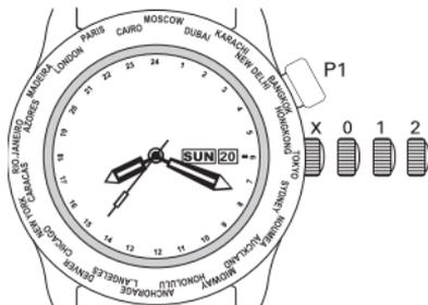
In position [2], turning the crown clockwise will advance the local time and the World Time disc. Turning the crown counter-clockwise will reverse only the local time; the World Time disc remains unchanged.
