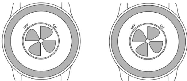
By locking the rotor of the automatic movement, the BALL Amortiser© shock-absorbing system reduces the risk of damage during high-impact activities.
