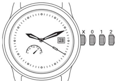
The Trainmaster Power Reserve features a power reserve indicator that displays the remaining power reserve on a hand. The indicator will turn counter-clockwise as the power diminishes. During manual winding or when the watch is worn, the reserve indicator will move clockwise.
