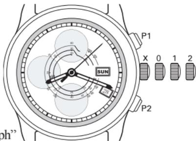
To compute the speed of a car over a certain distance, press the top chronograph button [P1] to start timing. At the end of the fixed distance, press the button again. If the time elapsed is 45 seconds, the second hand should point to the figure 80 on the Tachymeter scale. If the fixed distance is a kilometer then the car is traveling 80 kilometers per hour.
