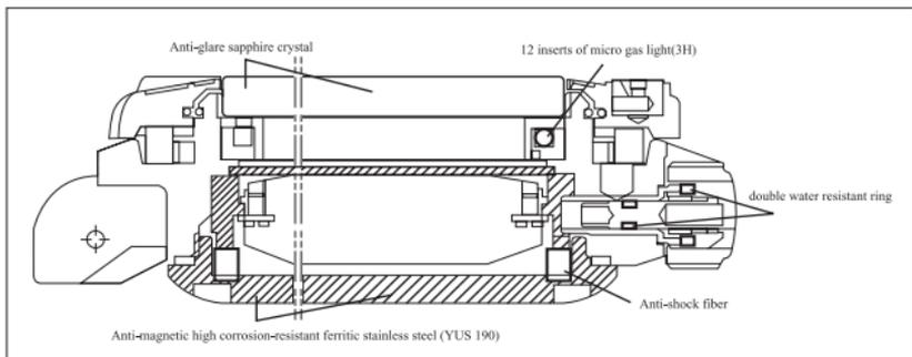
BALL case construction to protect against magnetic fields
