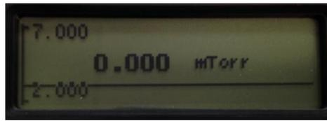
In this mode, the pump down graph is shown with a linear pressure scale that is fit to the pressure range of the data set. The height of the graph display is the pressure range of the data set in a linear scale (not log). The top left figure is the maximum value in this range, and the bottom left figure is the minimum value in this range.
