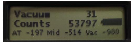
Press the circular arrow button to cycle through the calibration presets. Each function will capitalize when highlighted. Clear existing vacuum offsets by pressing the UP and DOWN buttons simultaneously; the number displayed next to the preset will reset to zero.
