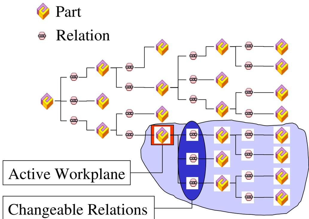
**Figure 46: Active workplane in the tree structure**
