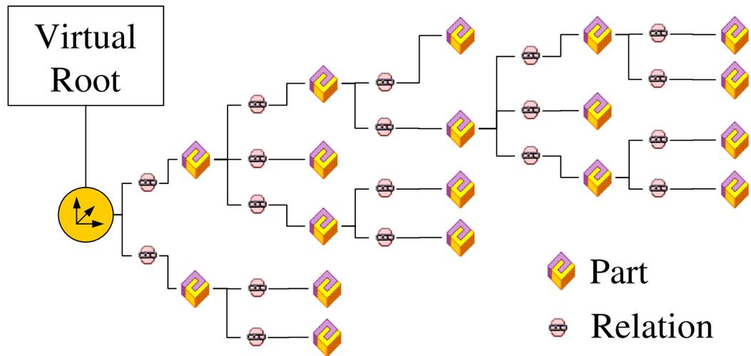
**Figure 45: Tree structure with several trees and a virtual root**
