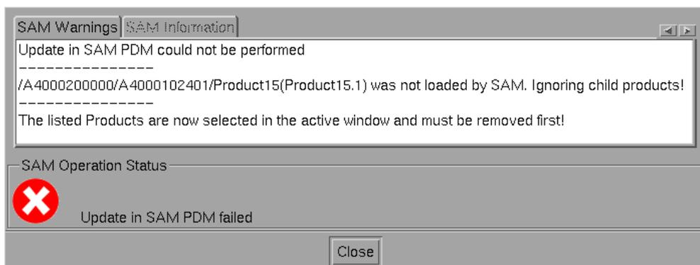
**Figure 57: Error messages at "Update SAM PDM" if structure is not consistent**
