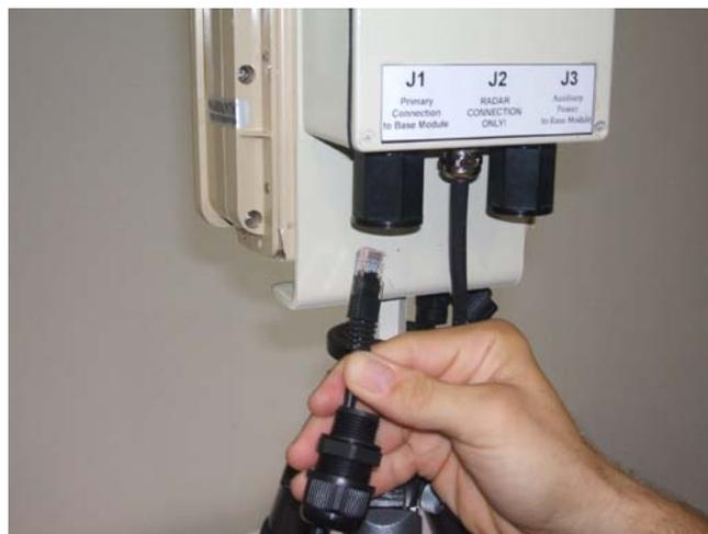
**Figure 3: Radar Remote Module CAT-5 Primary Connections (125m or less)**
