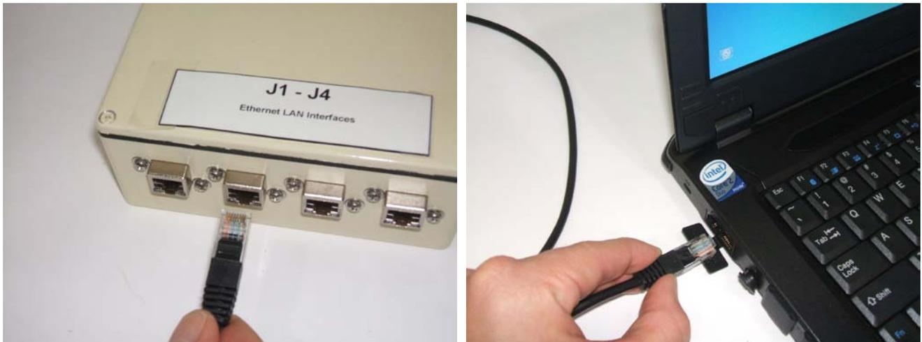
Figure 7: Connecting Radar Base Station to Computer
