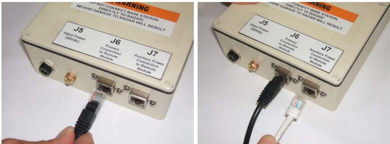
**Figure 5: Connecting Radar Remote Module to Base Station**
