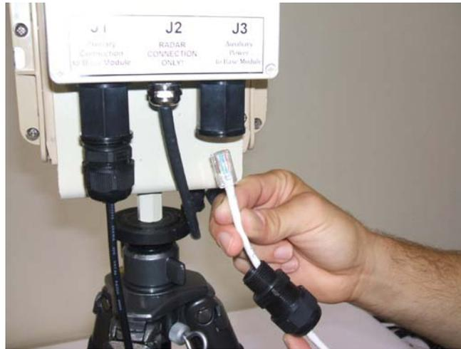
**Figure 4: Radar Remote Module CAT-5 Auxillary Connections (125m -450m)**
