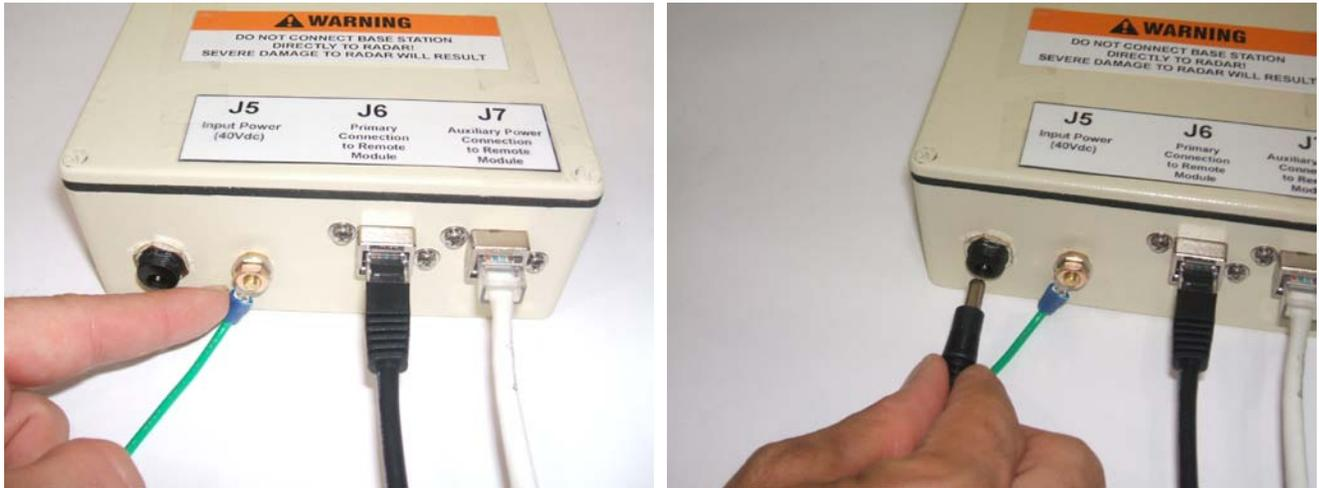
Figure 6: Powering Up the Radar Base Station
