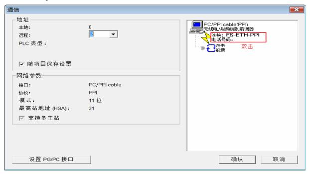
Select the "Radio / RF modem" and configure serial port parameters, choose no parity 10 bit mode.
