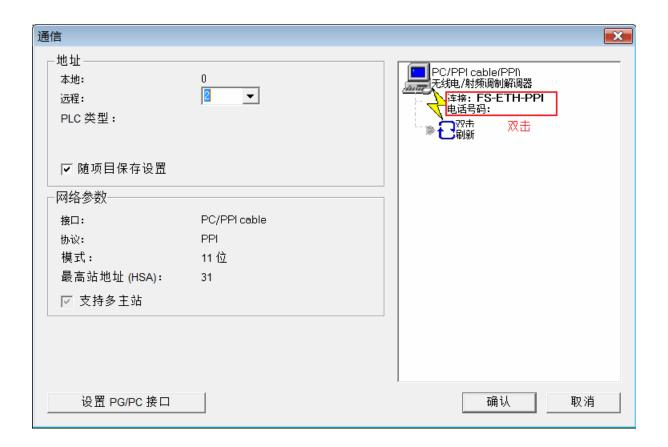
Select the "modem connection" and configure serial port parameters, choose even parity 11 bit mode.
