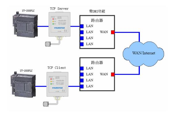
Two pcs S7-200PLC can achieve remote communication on the Internet via the FS-ETH-PPI, you need a router which supports dynamic domain name (DNS),in order to avoid the high cost of fixed IP address from the local telecom, and this router is very common now, please notice the instructions on the package when you purchase it.
