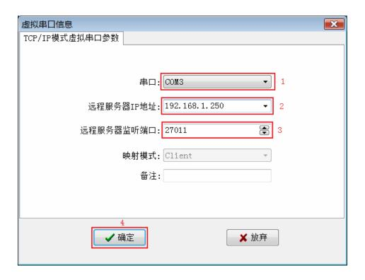
Click OK and exit the software and re-run VCOMM, the client side VCOMM will take the initiative to connect the server side with IP address 192.168.1.250, port number 27011, it will create a new serial port COM3 after establishing the connection, and it will appear in the Device Manager of the Windows system, then you choose this serial port in your application software, such as STEP7 Micro/WIN.
