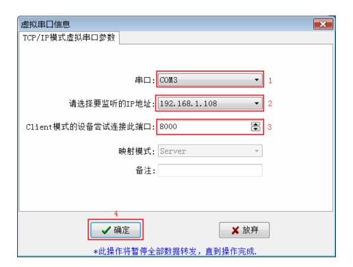
Click OK and exit the software and re-run VCOMM, server side VCOMM will accept as many as client side FS-ETH-PPI connections, and it's unlimited. A new serial port COM3 will appear on the PC after the connection is established. And this serial port will also appear in the Windows System Device Manager, then you can choose this serial port in your applications,like STEP7 Micro/WIN.
