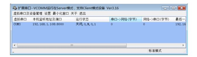
You can also set the FS-ETH-PPI as the server, set VCOMM as the client, but the router connected with FS-ETH-PPI need to have the DNS function, or you can use a PC connected to the router which is connected with the FS-ETH-PPI to run the peanut shell software to resolve the domain name. When the VCOMM software work as the client, you also could input the domain name directly in the remote server IP address, support DNS resolution.
