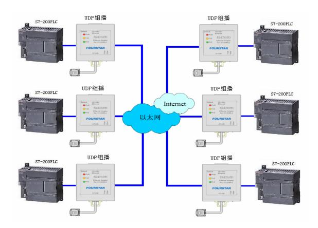
When multiple S7-200PLC need to exchange data each other, of course UDP multicast mode is the best working mode. Using UDP multicast can directly replace the original multi-point RS485 communication. But please notice that at this time the FS-ETH-PPI only supports S7-200PLC free port RS485 communication mode, do not support PPI,advanced PPI,Multi-master PPI communication protocol and MPI and profibus protocol.
