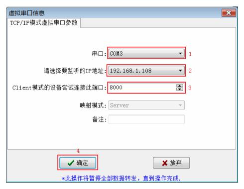
Click OK and exit the software and re-run VCOMM, the server VCOMM will wait the connection of client FS-ETH-PPI, then it will create a new serial port COM3 after establishing the connection, and it will appear in the Device Manager of the Windows system, then you choose this serial port in your application software, such as STEP7 Micro/WIN.
