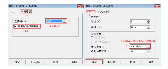
Click the "Communication" button to enter the communication settings, double-click "connection" to set the modem parameters.
