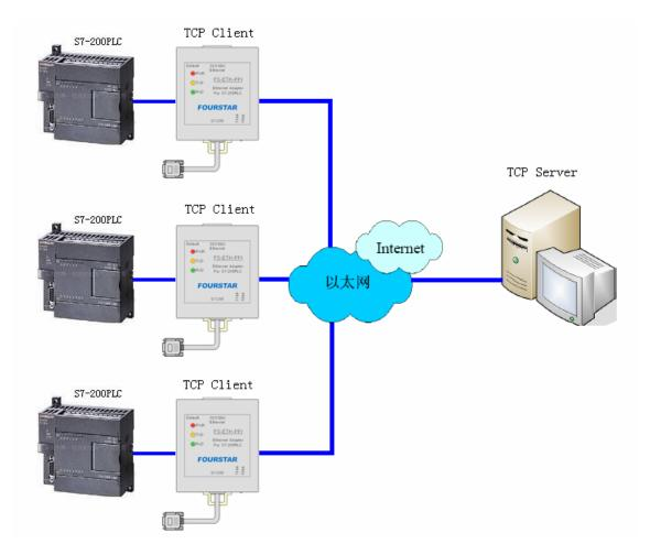
When multiple PLCs communicate with a PC via Ethernet, you need to set every FS-ETH-PPI connected with PLC as TCP Client, set the PC as the TCP Server, let every client FS-ETH-PPI takes initiative to connect the server PC. When VCOMM Virtual Serial Port Software work as TCP Server, it allows unlimited number of connected clients.
