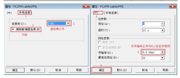
Click the "Communication" button to enter the communication settings, double-click "connection" to set the modem parameters.
